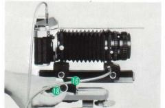
The assembly should be positioned with the lens side a little on the heavy side. Adjust the position of the tripod mount by turning the shift knob (18). Although mounting the assembly at its center of gravity would appear to be more stable, it can in fact often result in camera movement. A camera-heavy situation is definitely undesirable.
