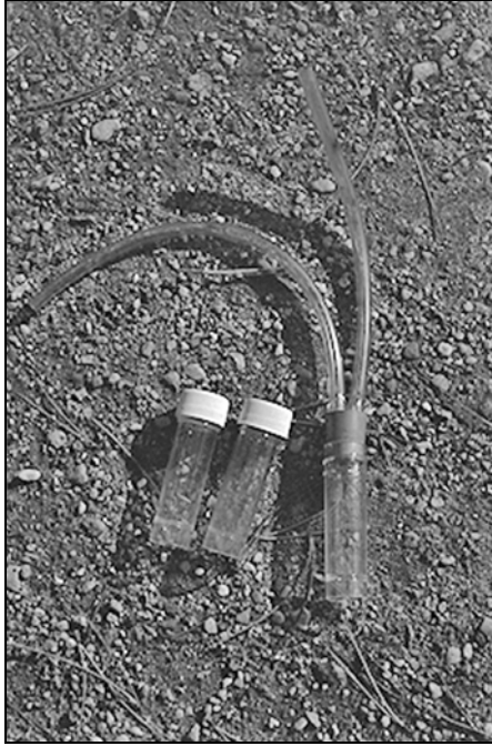
Figure 4: A pooter designed around a Sterilin™ universal sample tube
