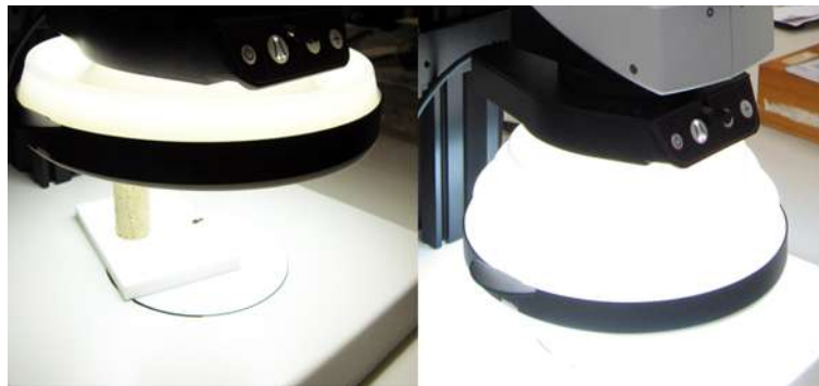
Figure 2 Leica lighting hood in action
