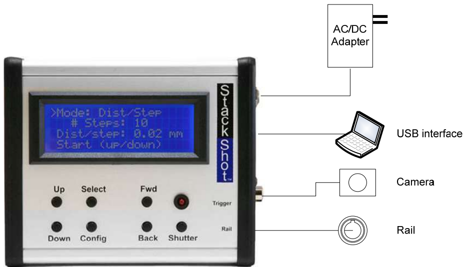
Figure 1 - Typical Connection Diagram
