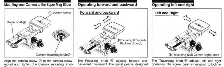
2. The lens should face forward to the Guide shaft (6) when mounting the camera.
