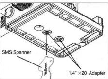
Both A and B camera screw mounts are fitted with 1/4"×20 adapters. If the tripod screw is 3/8" ×16 thread simply remove the adapters.
