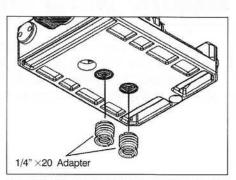
Adapter can be removed as shown in the illustration.
