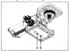
Use either A or B camera screw mounts when attaching the Super Mag Slider to the tripod. Choose the mount which offers better balance, this will depend on the position of the tripod screw.
