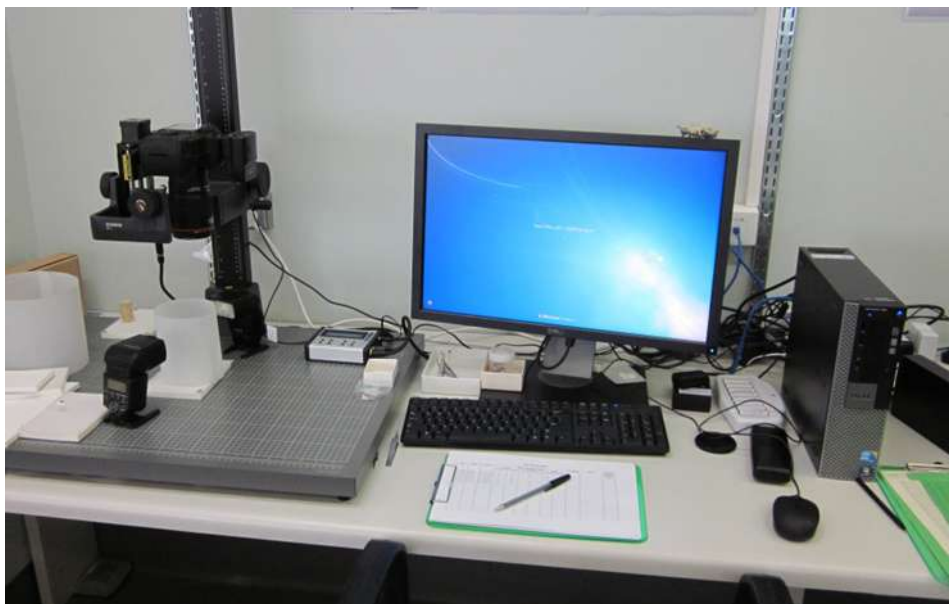
Figure 10 SAMA's adapted macrophotography system
