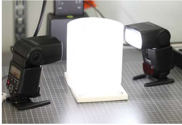
Figure 1 Wireless flash units diffused with tracing paper ring
