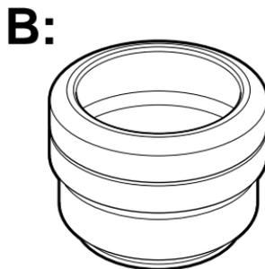
■ Attach the adapter to the lens that is on the camera.
