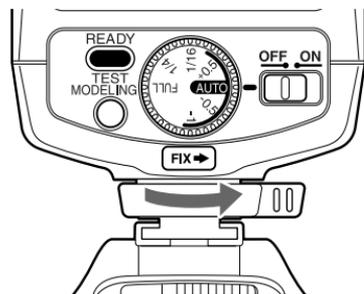
**2** Turn the locking lever of the controller away from [FIX →]. Loosen it so the flash shoe mounts easily.
